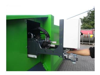
The APB 616 as well was developed with the advantage of linearly arranged cylinders. This results in higher power transmissions of about 15% compared to the scissor-like compaction system.
